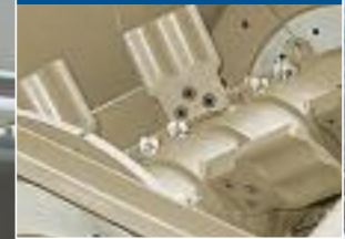
BOLT-ON WEARS FOR QUICK CHANGES
