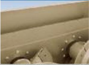
FULL WIDTH OVERFLOW WEIR
